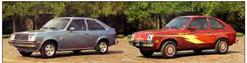
In this GM Styling photo, the Electrovette Concept is posed next to what appears to be a design prototype for the restyled 1979 regular-production Chevette. The Electrovette’s shortened wheelbase is apparent here.
