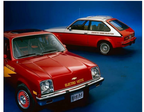
Chevrolet Electrovette Concept (foreground) and Chevette Turbo Injection. Both vehicles were based on the production Chevrolet Chevette. The Turbo Injection featured a turbocharged and fuel-injected version of the Chevette’s stock 1.6-liter engine. It made 100 horsepower—37 more than the standard mill.
