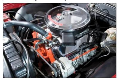
There were actually three 396 cubic-inch V8s introduced in early 1965, including the L78 for the Corvette and full-sized cars and the L37 for a special version of the Chevelle SS known
