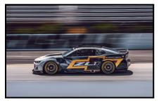
ZL1; A new transaxle that combines the transmission and rear gears into one package; The bottom of the car will be sealed with an underwing and rear diffuser for enhanced aerodynamics; A redesigned chassis features new front and rear bumpers with an energy-management system; Both the front and rear clips bolt on to the center section for easier serviceability and damage repair.
