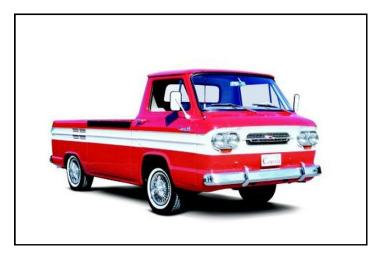
than Volkswagen's pickups, and could be had with Chevrolet's two-speed Powerglide, or a four-speed manual. The gross vehicle weight rating of 4,700 pounds meant that they could handle a payload of up to three-quarters of a ton.
